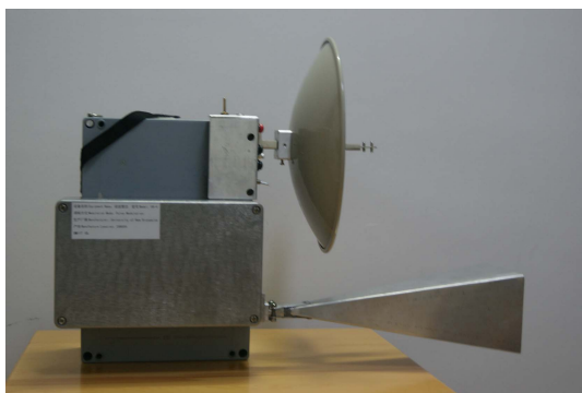
图2 便携式昆虫谐波雷达 (Gen IV) Fig. 2 Potable insect harmonic radar
